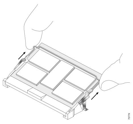
Figure 51 Remove Retaining Clip from Memory Module Socket
